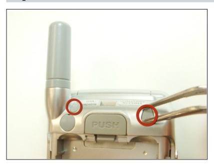
Use a push-pin or tweezers to pry both of the tear-shaped screw covers out of the top of the phone.
