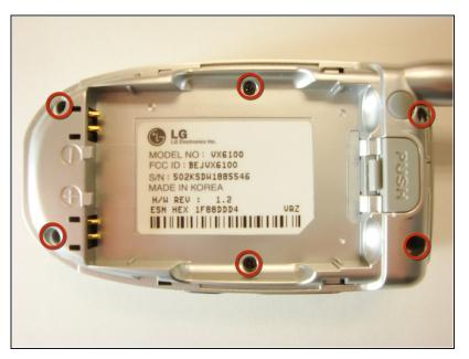
Use a Phillips #00 screwdriver to unscrew the six case screws from the back of the phone.
