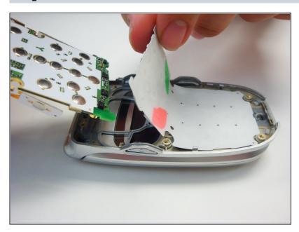
Gently lift up on any edge of the white keypad to remove it from the phone case.
