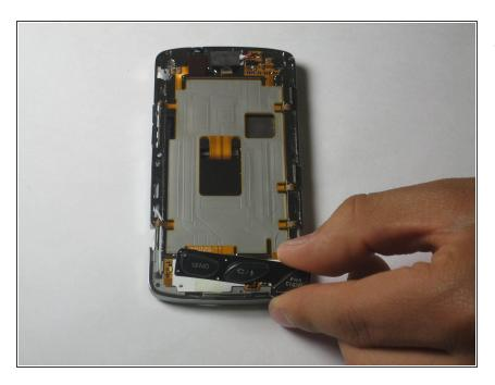
With the phone still facing upwards, identify and remove the three buttons at the bottom end that say "Send", "Clear", and "End." They should come off easily.
