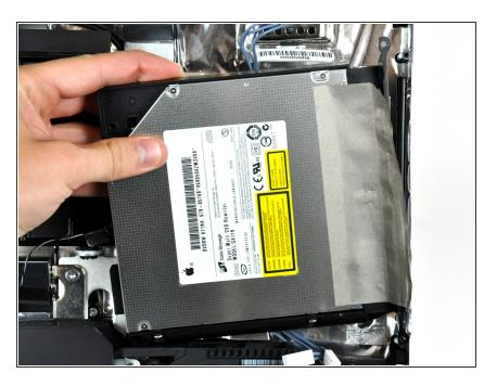
• Lift the left edge of the optical drive slightly and pull it away from the right side of the rear case.
