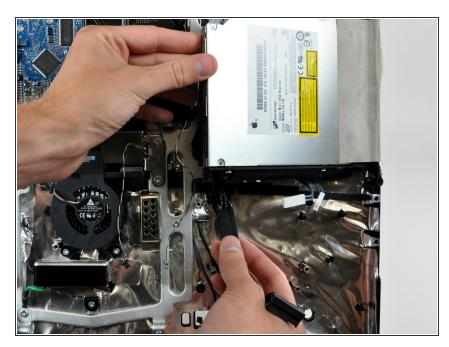
Peel the optical drive data cable off the adhesive securing it to the rear case and remove it from your iMac.
