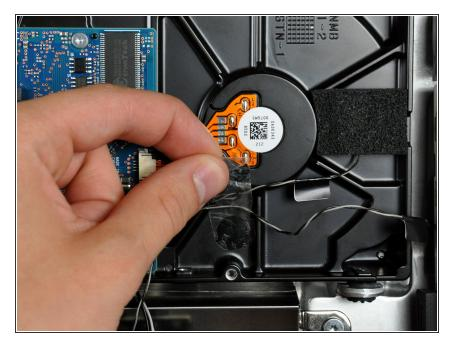
If necessary, remove the piece of tape holding the thermal sensor wires to the hard drive.
