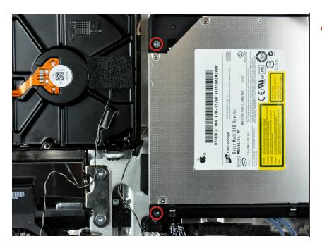
Remove the two T10 Torx screws securing the optical drive to the rear case.
