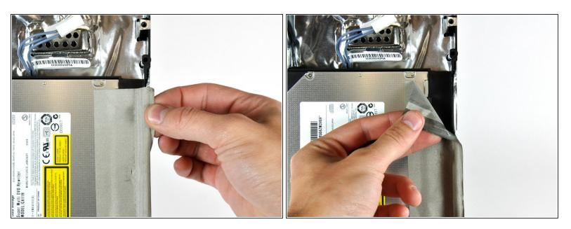
• Peel the strip of EMI tape off the edge of the rear case.
