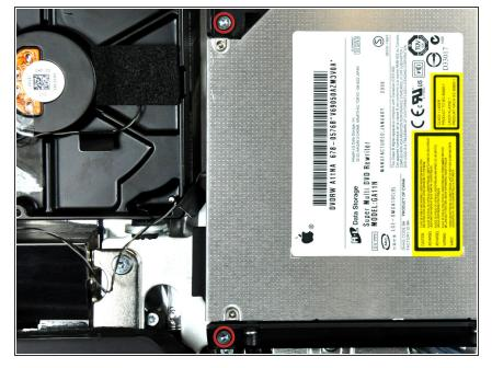
Remove the two T10 Torx screws securing the optical drive to the rear case.
