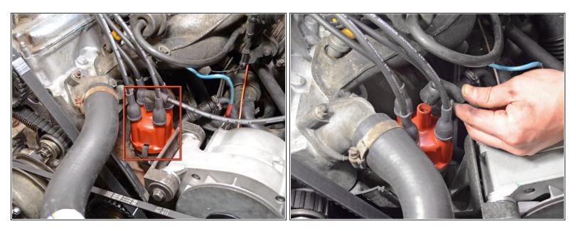
(i) The distributor cap is located next to the engine and has all of the spark plug wires connecting to it.
