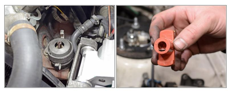
The distributor rotor is keyed, which means that the new rotor will only go on in one orientation.
