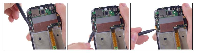
• Use the pointed edge of a spudger to work the ZIF cable out of its connector.
