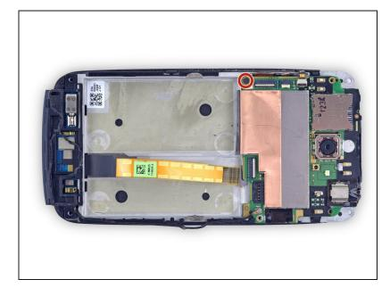
• Remove the 3.15 mm Phillips #00 screw from the motherboard.
