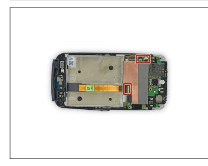
• Repeat the procedure from steps 19 and 20 to remove the cables from the remaining ZIF connectors.
