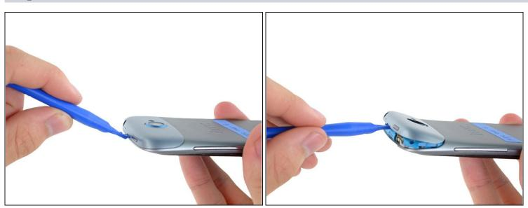
• Starting at the groove near the headphone jack, use a plastic opening tool to lift the top casing.
