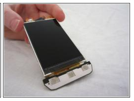
Unhook the LCD from tabs on the bottom using the plastic opening tool.
