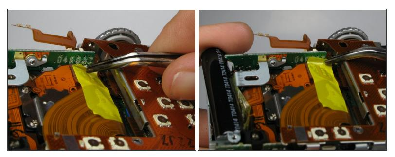
• Carefully remove the yellow piece of adhesive tape connected to the motherboard.
