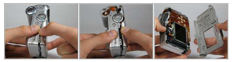
• Separate the back casing and front casing of the camera using your hands.
