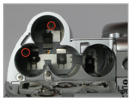
• Remove the two 4.1mm screws at the bottom of the battery flap.
