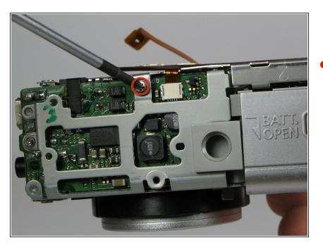
Remove 2.5mm the screw in the silver housing on the bottom of the camera. This screw is holding the back panel in.
