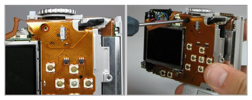
Remove the 3.4mm screw inside a deep hole on the back copper panel beneath the circular mode switcher.
