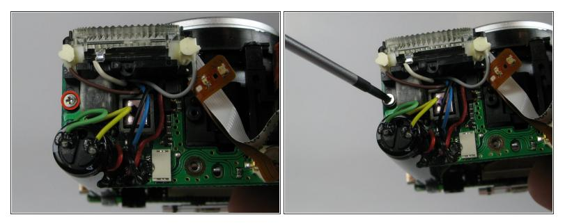
• Remove the 3.5mm screw found near the capacitor and the flash unit.
