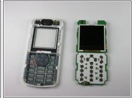
Put the red casing aside and remove the motherboard from the front casing of the phone by carefully dislodging it from its two clips near the top of the phone.
