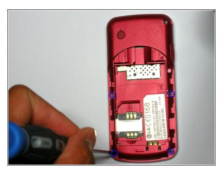
Remove the four screws along the edge of the phone body, as shown in the picture to the left.
