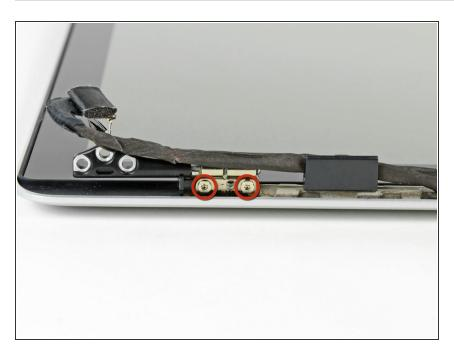
Remove the remaining two 5.2 mm
