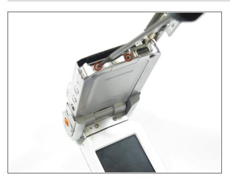
Remove the two screws (2.2mm Philips) indicated.
