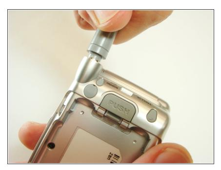
Hold the phone upright and firmly twist the antenna counter-clockwise until it becomes loose. Once loose, pull upwards to remove the antenna from the phone.
