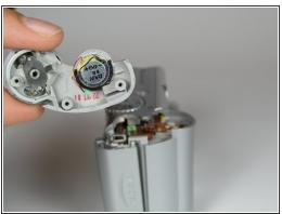
Using a pair of tweezers, grab the plug that connects the speaker to the camera and gently pull it out.
