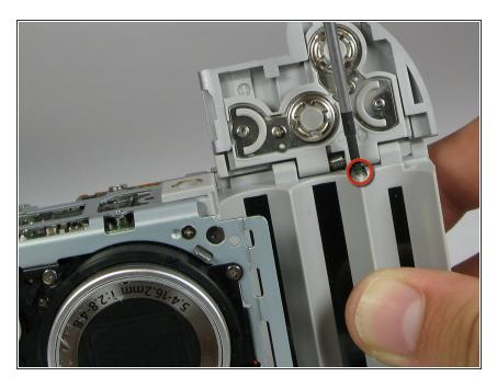
Remove the 4.2mm screw directly under the battery flap.
