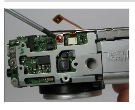
Remove 2.5mm the screw in the silver housing on the bottom of the camera. This screw is holding the back panel in.
