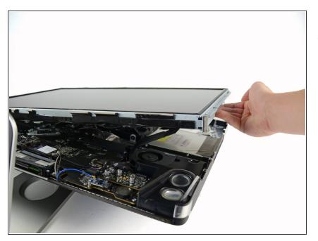
• Lift and remove the display panel from the device.
