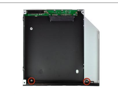
Remove the two 3.0 mm Phillips screws securing the faceplate to the optical bay enclosure.
