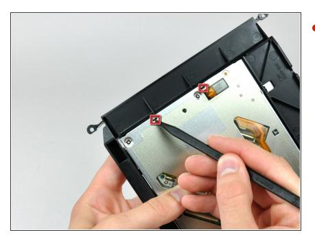
• Use the tip of a spudger to press each of the optical drive bracket tabs out of their slots on the bottom of the optical drive.
