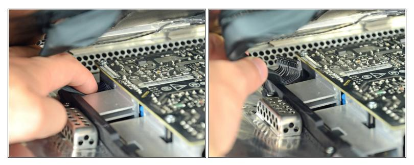
• While still holding the display panel up, use two fingers to firmly push down on the power supply cable connector from its socket.
