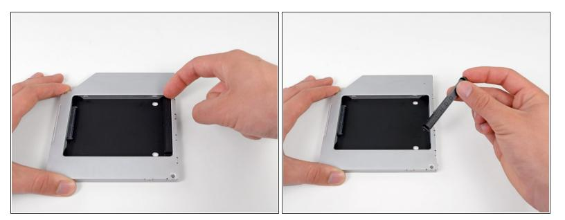
Remove the plastic positioner from the optical bay hard drive enclosure by pressing in on one of the clips on either side and lifting it up and out of the enclosure.
