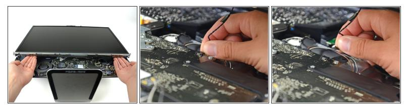
• Place your hands on either side of the bottom of the display panel, and lift it up enough that you can reach the connectors inside.
