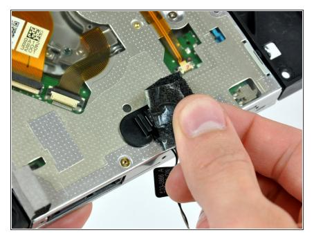
Remove the piece of foam tape covering the optical drive thermal sensor.
