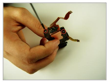
Locate and unscrew the two 3mm screws on the bottom of the black lens box with the JIS #0 screwdriver.
