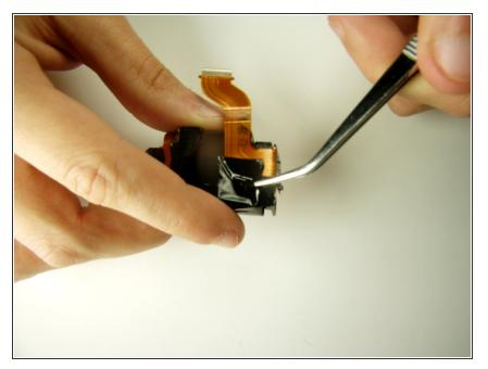
• With the tweezers remove the black tape to detach the chip from the lens box.
