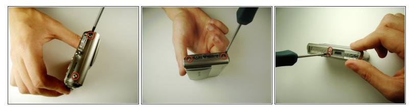
Locate and remove the 3mm screws on the bottom and sides of the camera with a JIS size #0 screwdriver.
