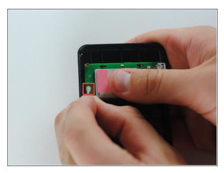
To disconnect the antenna, pull up on the antenna's connection to the circuit board until it pops off.
