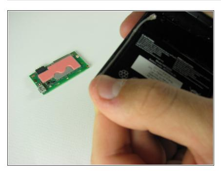
Simply pick up the circuit board with your fingers and remove it from the case.
