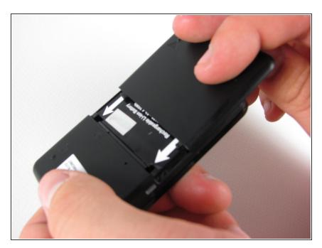
Remove the rear cover by pressing down on the cover and pulling it away from the device.
