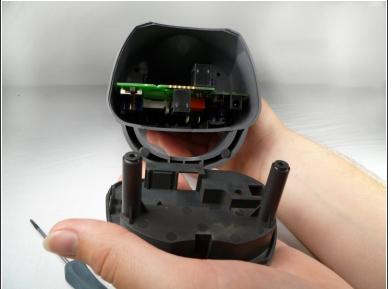
Using a #0 screwdriver, remove the two 2.50mm screws.
