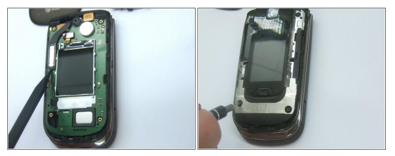
• Take the new logic board and connect all the parts you just disconnected to their correct locations.
