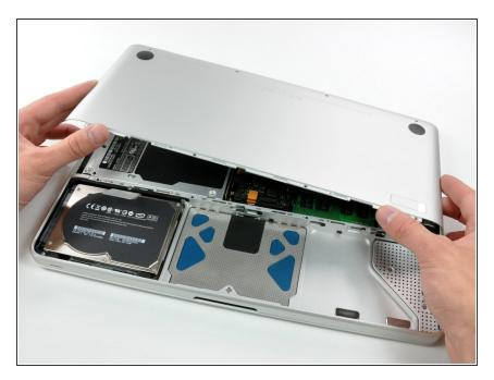
Using both hands, lift and remove the lower case off the upper case.
