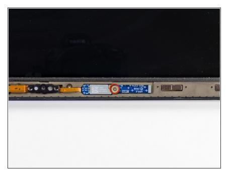
Remove the single 3 mm Phillips #00 screw securing the Bluetooth board to the display assembly.
