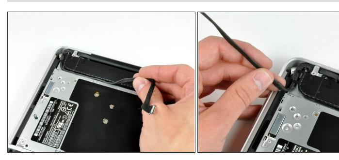
De-route the camera data cable from the channel in the optical drive.
