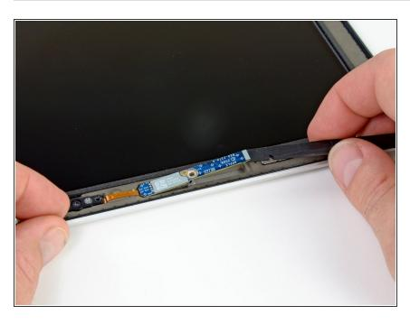
Use the flat end of spudger to flip up the Bluetooth board from its recess within the display assembly.
