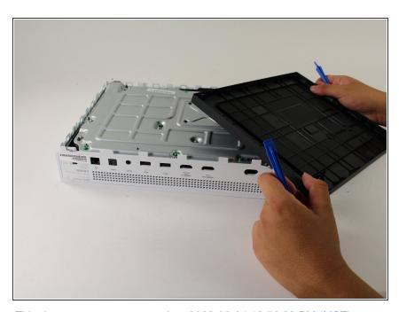
Once all of the clips are opened, remove the bottom part of the case.
