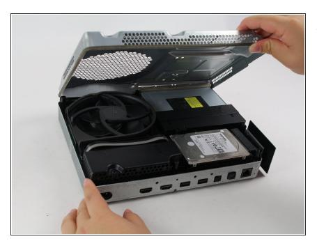
To access the hardware within the casing, you can pop and lift the top panel of the casing. It should come right off.
