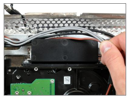
De-route the bundle of power supply cables from behind the hard drive bracket.
