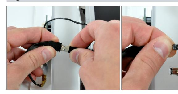
Disconnect both the camera and microphone cables.
