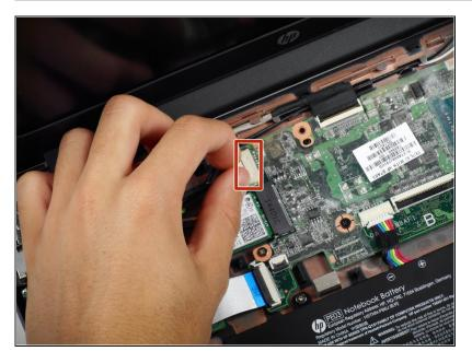
Gently remove the charging port's slide-out connector from the motherboard.
