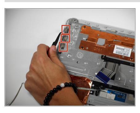
Using tweezers, pull back the three metallic-colored pieces of tape near the top left corner of the keyboard mount.
