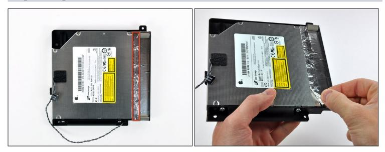
• Peel back the portion of aluminum tape highlighted in red, leaving the rest attached to the black plastic optical drive bracket.
