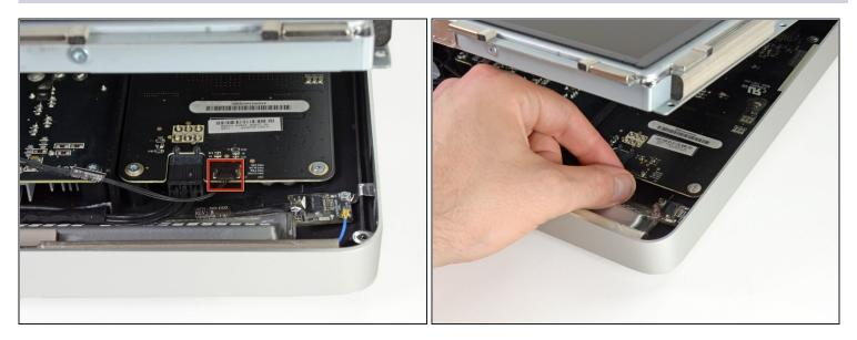
• Using your fingers, carefully pull the vertical sync cable out of its socket on the LED driver board near the top left corner of your iMac.
