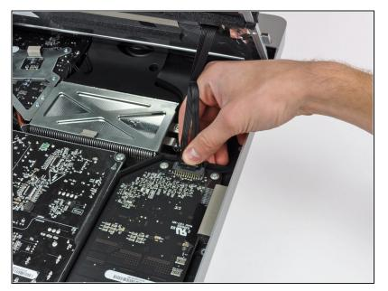
Rotate the display out of the outer case enough to disconnect the LED backlight power cable from the LED driver board.
