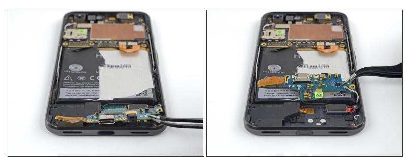
• Using tweezers, lift the daughterboard up and flip it over onto the battery.
