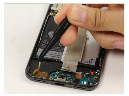
Using tweezers, lift the contact pads located to the left of the daughterboard.
