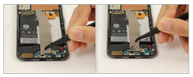
Use tweezers to lift up the silver strip at the top of the daughterboard, and peel it back to expose the connector underneath.
