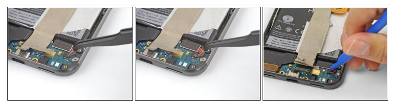
(i) The vibration motor is connected to the daughterboard with a small socket connector.
