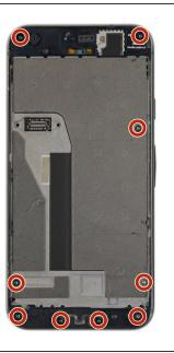
Use a T5 Torx driver to remove the nine 3.5 mm screws securing the midframe.
