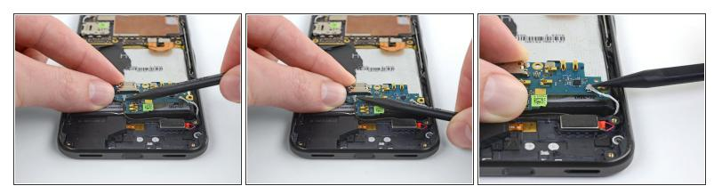
Use a spudger to pry up the black and white <u>coaxial cables</u> attached to underside of the daughterboard.
