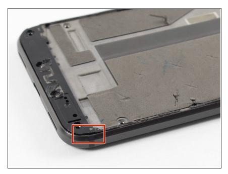
• Wedge an opening pick into the notch that is located at the bottom right corner of the phone.
