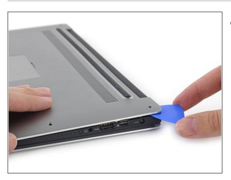
Use opening picks or a plastic pry tool to pry open the case clips, beginning from the back edge.
