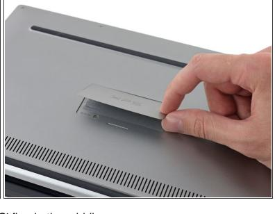
• Use a plastic opening tool to pry open the 'XPS' flap in the middle.
