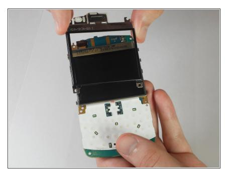
Unhook the screen frame from the small tab at the top of the motherboard.
