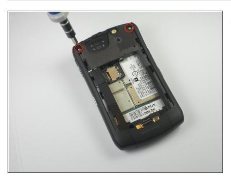
Remove the two top screws using a T5 Torx screwdriver.
