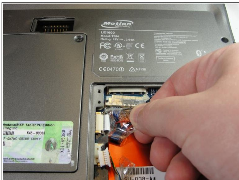
**⚠ Caution:** do not pull on the wires, instead pull from the plastic connectors.
