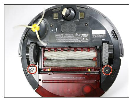
Remove the two 10mm screws holding the back plate in place using a Phillips #2 screwdriver, and then remove the plate from the device.
