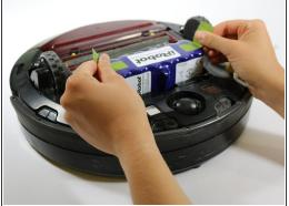
Remove the battery panel and 10mm screws with a Phillips #2 driver and then take the battery out
