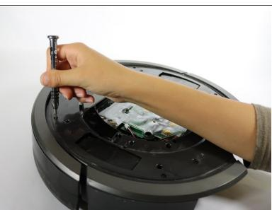
Using a Phillips #0 screwdriver, remove the six 10mm screws holding the black panel in place.
