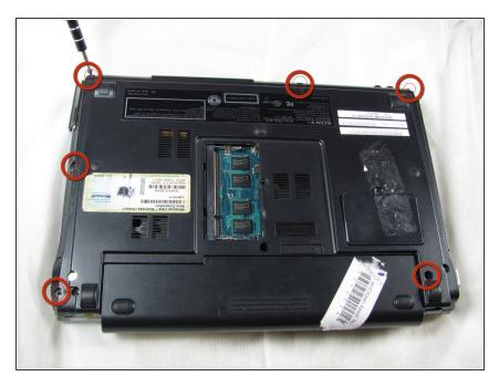
Flip computer over and remove the 6 screws.
