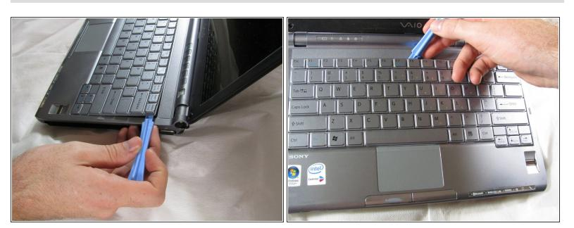
• Use a plastic opening tool to gently lift the keyboard at a corner.
