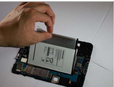
You can now safely remove the battery from the device by lifting it from the paper flap.
