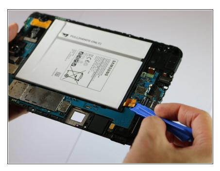
Remove the cable that connects the battery and device using the plastic opening tools.
