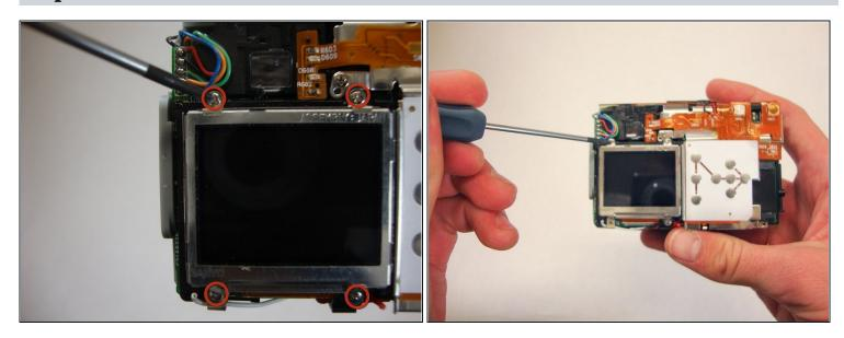
• Using a Phillips #00 remove the four 4.40 mm screws that secure the LCD screen to the frame.
