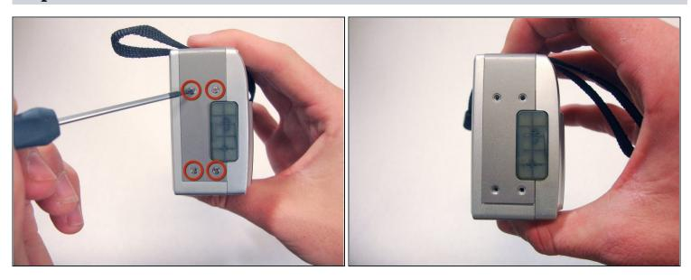
• Remove the four 4.7 mm screws on the left side of the camera.
