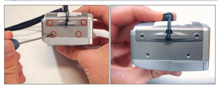
• Remove the four 4.7 mm screws on the opposite side of the camera.
