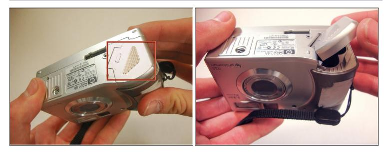
• Slide the bottom cover in the direction of the arrow to open it.
