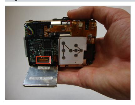
Allow the LCD screen to flip down. This will expose the electric strip that connects the screen to the camera.
