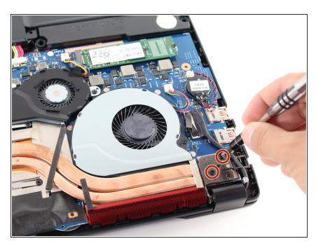
Using a Phillips #1 screwdriver, remove the two 6 mm screws that hold the hinge.
