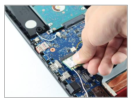
Disconnect the chip from the motherboard by pulling it gently toward the laptop hinges.
