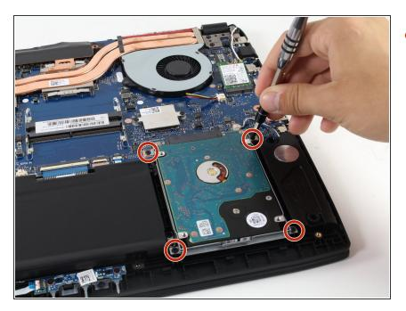
Using a Phillips #1 screwdriver, remove the four 4 mm screws holding the hard drive.
