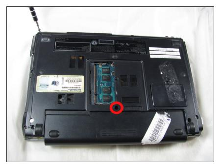
Take out the screw in the center of the computer.
