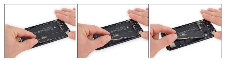
• Lift the battery connector end of the logic board and pull it up and out of the rear case.
