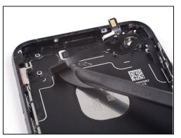
Continue to move the blade of the halberd spudger underneath the power and volume control cable.
