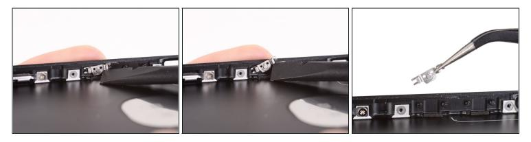
• Repeat the procedure to remove the second volume button bracket.
