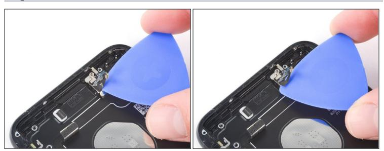
Moving from power button side of the phone, use an opening pick to separate the adhesive holding the antenna flex cable to the rear case.
