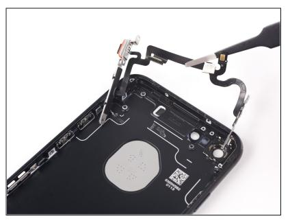
• Remove the power and volume control cable.
