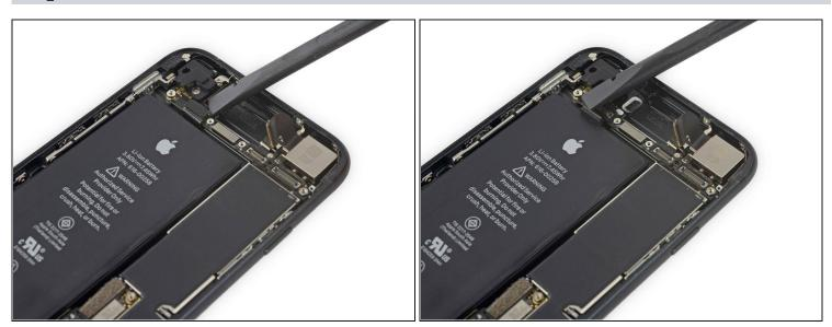
• Use the flat end of a spudger to disconnect the upper cable connector.
