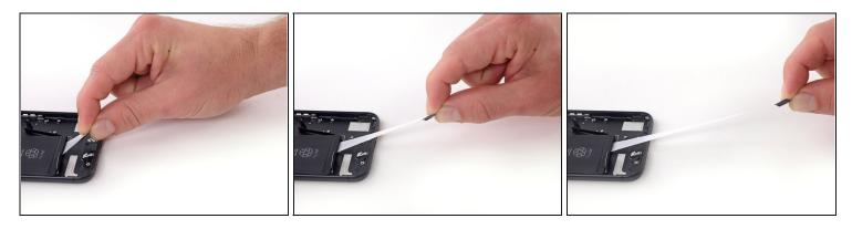
Try to keep the strips flat and unwrinkled during this procedure; wrinkled strips will stick together and break instead of pulling out cleanly.
