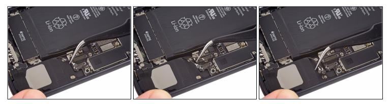
• Use tweezers to gently derout the antenna cables from the metal bracket on the logic board.
