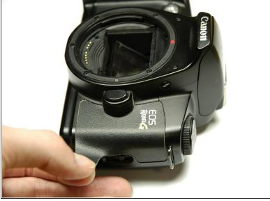
Using your finger, peel back the textured grip so the components are separated.
