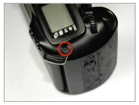
Using a #00 Phillips screw driver, unscrew the one 5.7 mm Phillips screw located next to the LCD screen.
