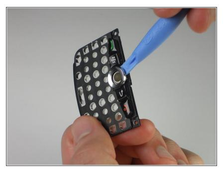
• Use a plastic opening tool to pry the trackball housing from the keyboard housing.
