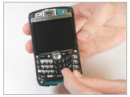
• Lift the flexible keypad away from the device. It should come off easily.
