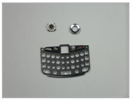
• Remove the trackball from the silver trackball housing by hand.
