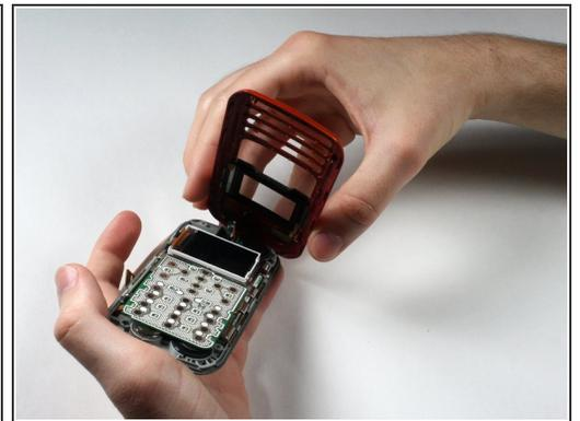
**⚠** Be careful while breaking the adhesive connecting the speaker and the casing in the following sub step so that you do not tear any wires.
