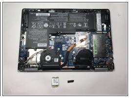
• The WiFi Card should be unbound from the surface. Carefully remove the card from the laptop by puling away from the socket.
