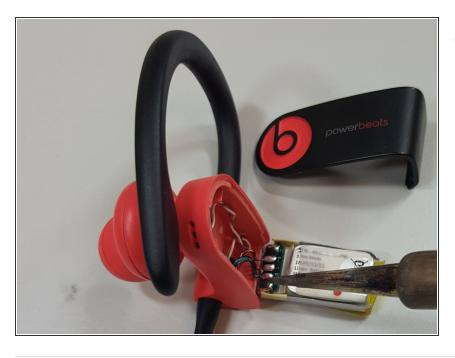
Use a soldering iron to desolder battery connection to remove battery and replace with new one.
