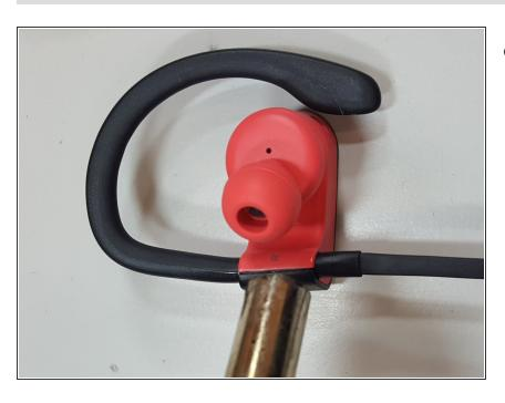
Use a heat gun with temperature set to 140 F for about 2-3 minutes and heat the casing where it attaches together as seen in the picture.
