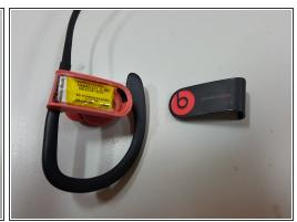
• After heating for about 2-3 minutes, separate the housing using a pry tool as seen in the pictures.
