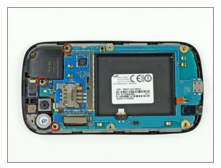
Remove the three Phillips screws securing the motherboard to the front display assembly.
