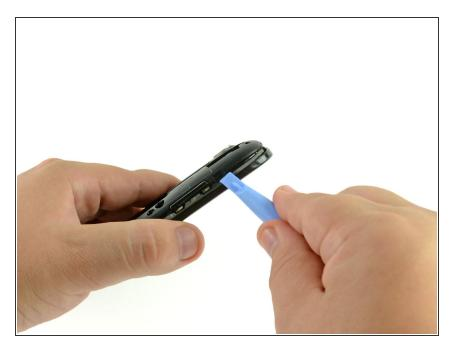
Insert and pry the plastic opening tool to release the final clip securing the rear inner frame to the inner assembly.
