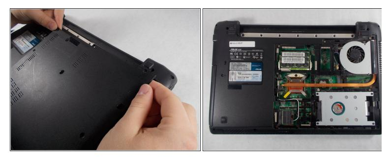
• Slide the back panel away and remove the panel.
