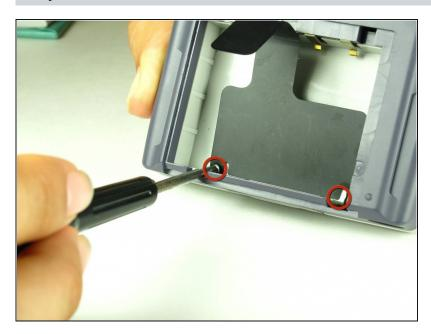
Use the Phillips #00 screwdriver to remove the two screws located inside the battery compartment.
