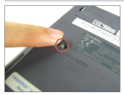
Slide the small switch on the back to "MAIN".
