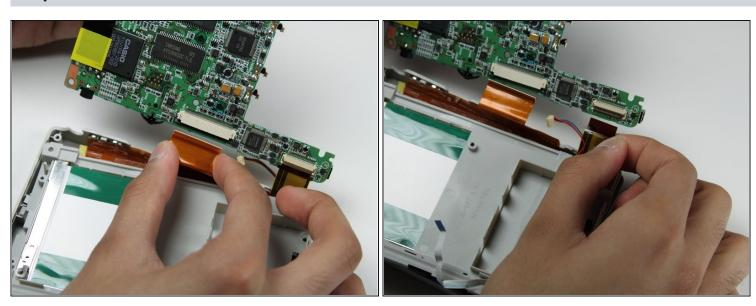
• Locate the two ribbon cables on the motherboard. Select one to remove first and then pinch either side of it and pull out to remove the ribbon cable. Do the same for the second.
