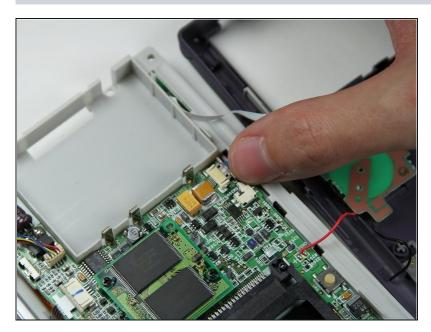
Locate the small grey ribbon cable towards the bottom of the device. It should be located above the battery slot. Pinch both sides of the ribbon cable and pull it out.
