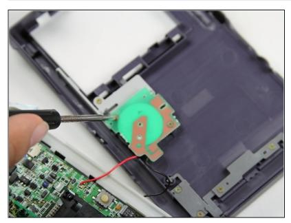
Use the Phillips #00 Screwdriver to remove the two screws from the green circuit board on the back case.
