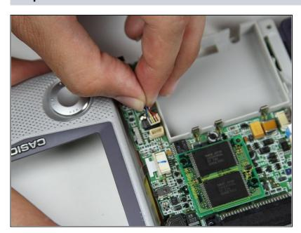
Locate the multicolored wire on the motherboard near the battery compartment. Pull on the wire by the base and lift to remove.
