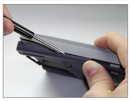
Use a spudger or opening tool to separate the two halves of the case.
