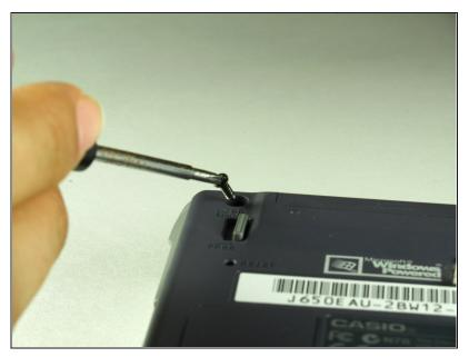
Use the Phillips #00 screwdriver to remove the two screws near the top of the device.
