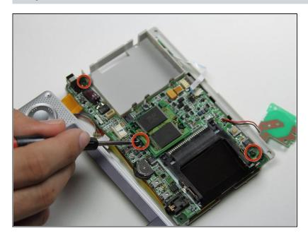
Remove the the three screws on the motherboard that are shown using the Phillips #00 Screwdriver.
