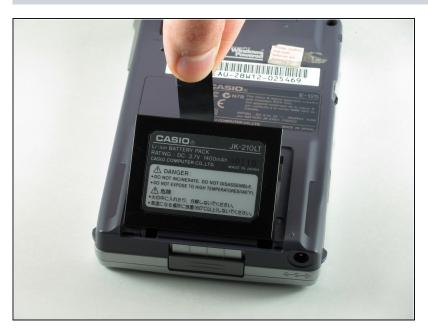
• Pull the black tab to remove the battery.
