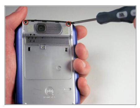
Using the #00 Phillips screwdriver, remove the two 9mm screws on the top corners of the device.
