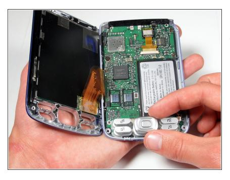
Lift the control pad buttons off of the motherboard. To reassemble your device, follow these instructions in reverse order.
