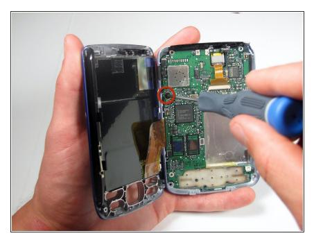
Unscrew the single 3.5mm screw attaching the motherboard to the case with a #00 Phillips screwdriver.
