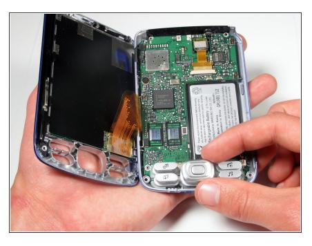
Lift the control pad buttons off of the motherboard.
