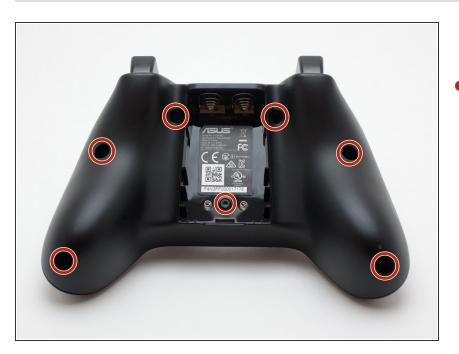
Remove seven 7mm T7 screws on the bottom of the controller.
