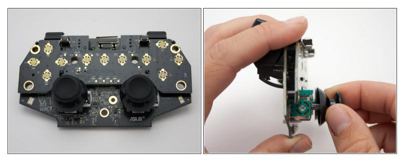
Now back to the logic board. Flip the board so the joysticks are facing you. Firmly pull each joystick straight out, away from the board, to remove.
