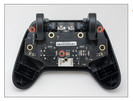
Remove three 7mm T7 screws that fasten the logic board to the top half of the controller.
