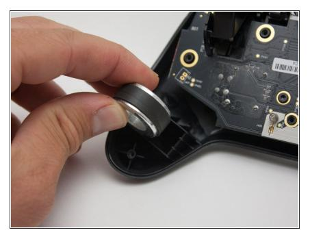
Now you can start disassembling the inside! First take the two weights out of their slots at the bottom of the controller (I know, kind of underwhelming, but you gotta start somewhere).
