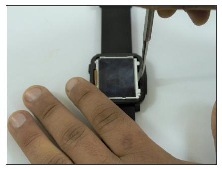
• Insert metal spudger into the side of the screen shown in the picture.
