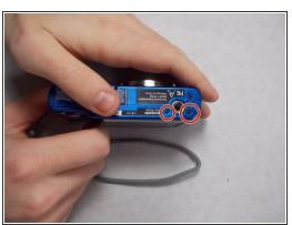
Remove 5 screws attached to the back case using a 00 Phillips head screwdriver.
