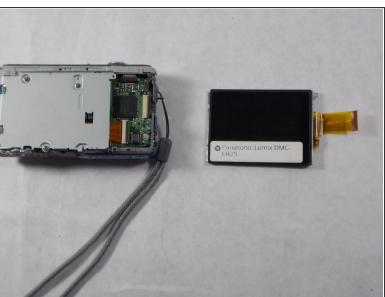
• One of the ribbon cables will be housed behind the screen and the other will be under the panels. Gently pull each free from the housing and remove the screen.
