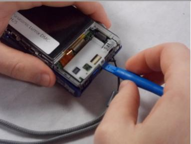
Access the ribbon cables by removing the green button receiver panel using a plastic opening tool. There is a white panel beneath. Carefully remove this using a plastic opening tool. The white panel may require some elbow grease to get it off, and the panel may make a snapping sound as it comes off.
