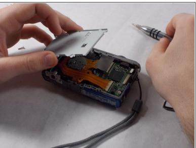
Under the screen is a silver panel. Remove three screws using a 00 philips screwdriver and take the plate off.
