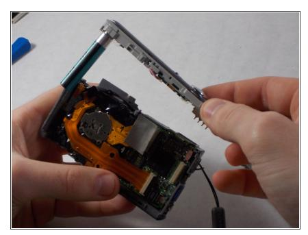
Remove the silver panel with the buttons and flash battery from the top of the camera. The silver tripod socket may fall out. Do not be alarmed and don't put it back in.
