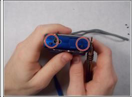
• Remove four screws on the front case using a 00 Phillips head screwdriver. Two will be on the side with the camera strap, one on the bottom, and one on the side opposing the camera strap. They will be in pairs, one screw holding the front case and one screw holding the back case.
