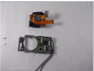
Gently remove the lens assembly. It should slide out cleanly.
