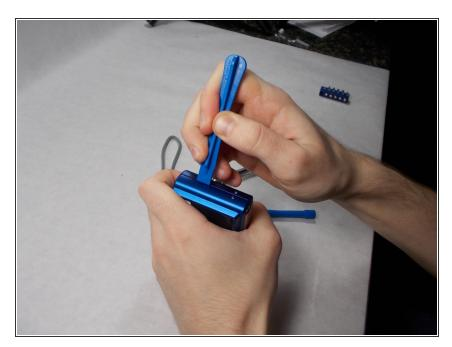
Using a plastic opening tool and your hands, pull the front case loose from the camera.
